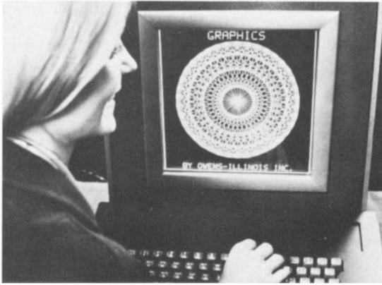
**Figure 5** Graphic display on a 21.6 cm (8.5 in) Owen-Illinois AC panel having  $512 \times 512$  lines with a resolution of 24 lines/cm (60 lines/inch)
