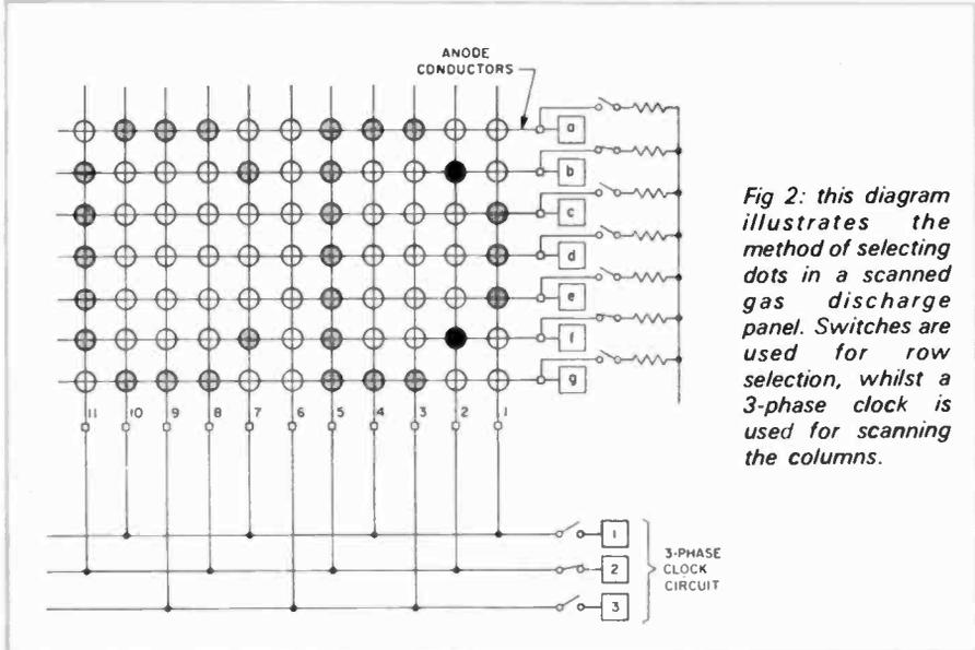
Fig 2: this diagram illustrates the method of selecting dots in a scanned gas discharge panel. Switches are used for row selection, whilst a 3-phase clock is used for scanning the columns.
